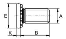
Head diameter E= 12.5Head height K +/-0.02 = 1.75Hole diameter +0.1= 8Length B +/-0.4= 20Male thread A= M8Min distance to edge= 12.5Tightening (N m)= 25.0
